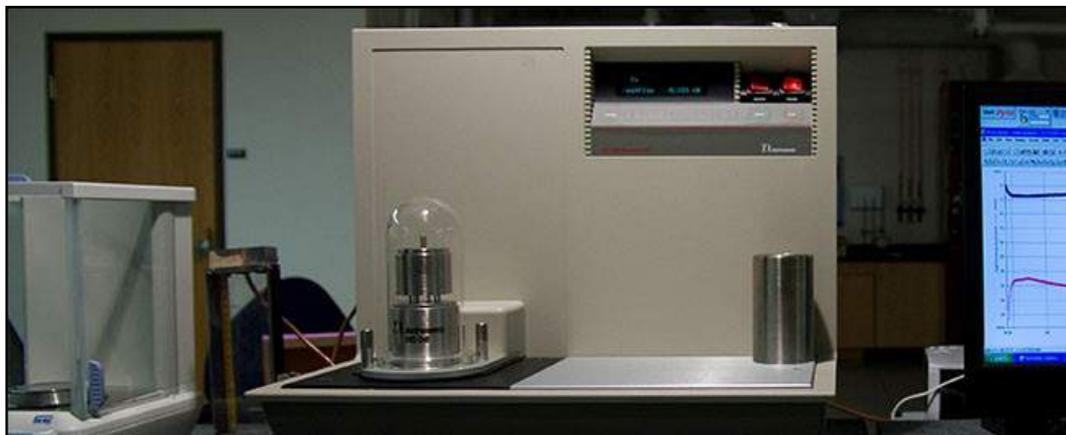
**Figura 3.15** – DSC 2920 TA Instruments.
